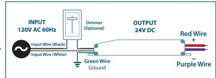
For smooth dimming 8W minimum load is required
